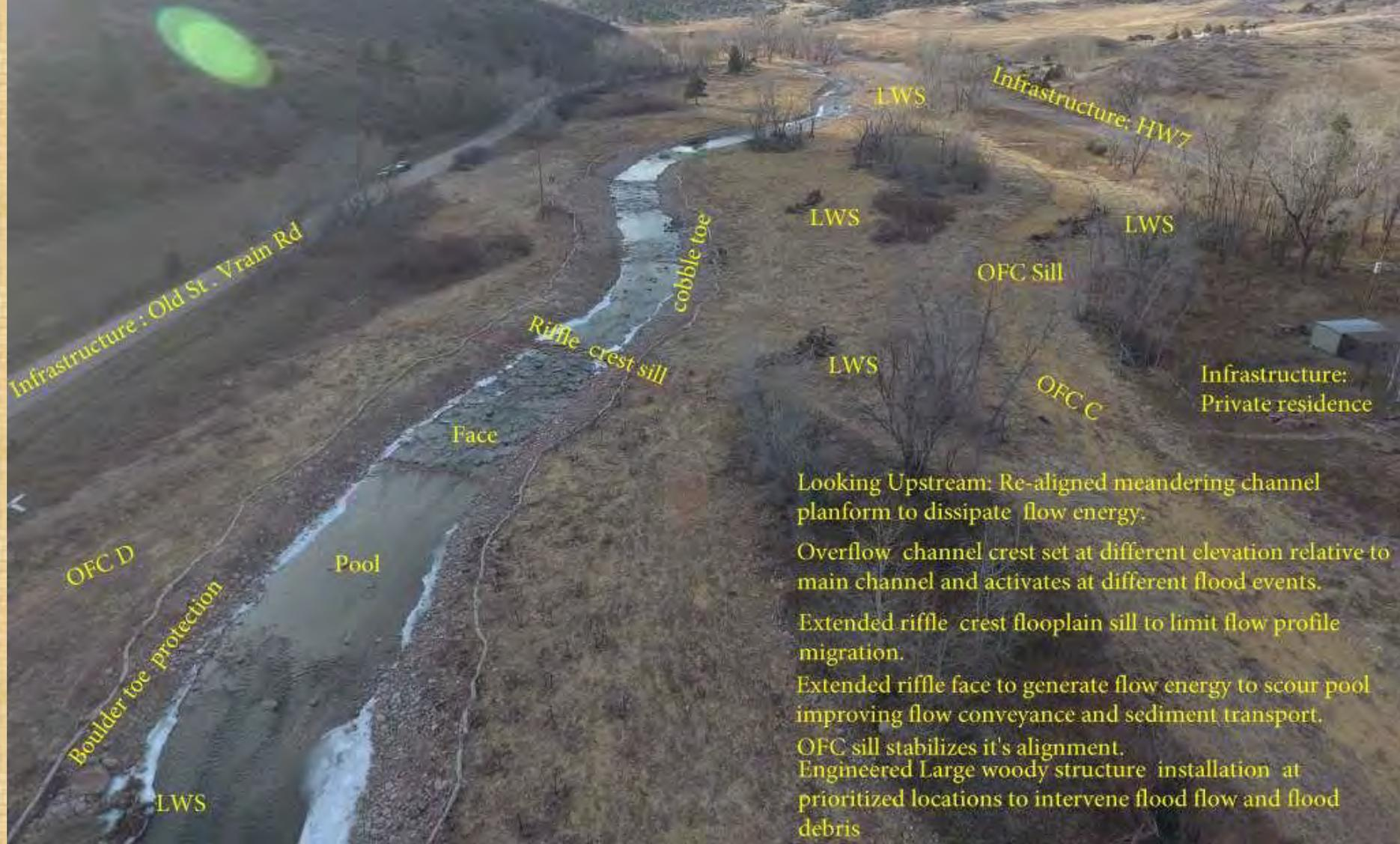
Looking Upstream: Re-aligned meandering channel planform to dissipate flow energy.
