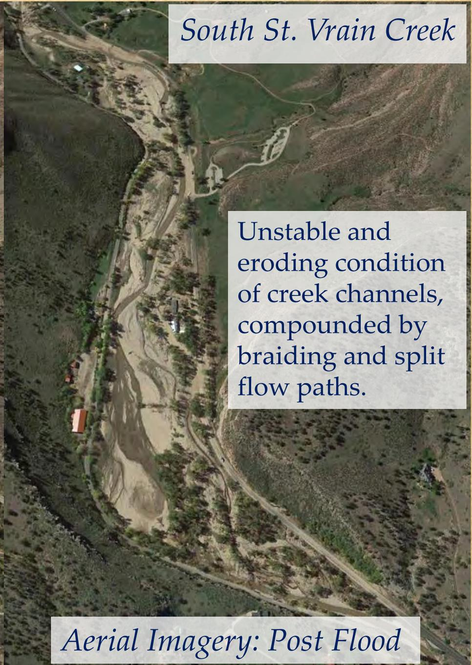
Unstable and eroding condition of creek channels, compounded by braiding and split flow paths.
